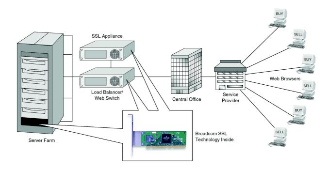
Broadcom's **SSL800** accelerator adapter is a complete high-performance SSL accelerator designed to accelerate the public-key cryptographic functions of SSL, thereby freeing the host CPU. This results in a dramatic improvement in the overall performance of the host system, drastically reducing CPU utilization and enabling additional CPU bandwidth for other value-added services and features.
